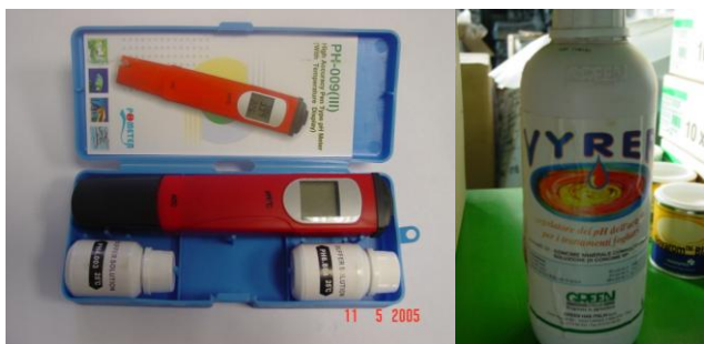
slika 6: pH meter v kompletu s pufrom 4,0 in 7,0
