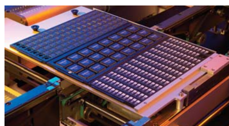
Area for 3 JEDEC trays on the dual heads machine, without reducing the feeder capacity
