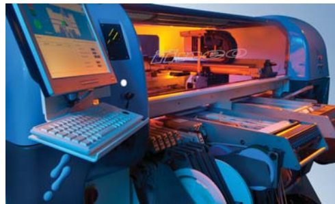
Placement head(s) are fitted with rotary turret head(s) with 8 or 12 pick ups.
