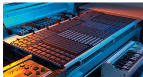
Huge area for 10 JEDEC trays on the single head machine, without reducing the feeder capacity
