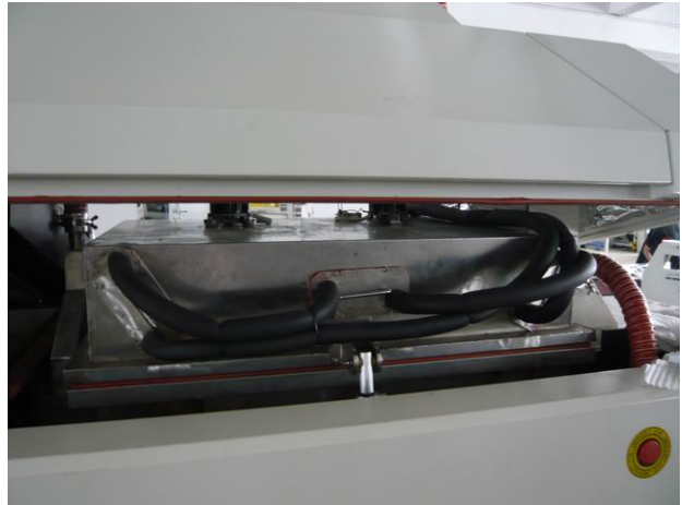
Cooling zone supplied with cold water by chiller
