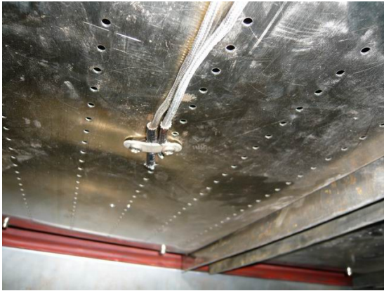
Dual thermocouple in each zone One for PC control, another for safe limiter
