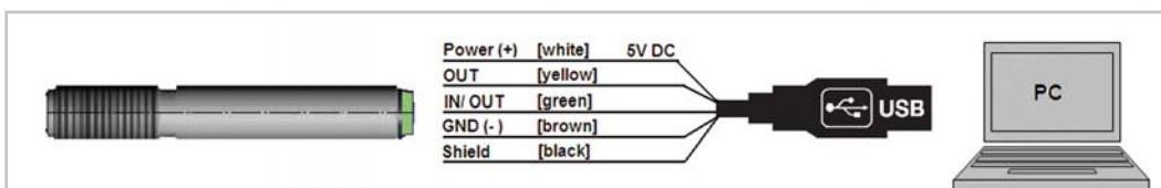
Device with simultaneous analog & digital operation with complete parameterization possibility via software
